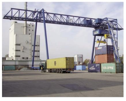
One thing applies to all three Barge Servers: the slewing trolley has double-winch equipment which can be turned around by approx. 305 degrees. It can be moved carefully and precisely to any container position. The driver can always keep an eye on what is going on from the integrated cabin.
