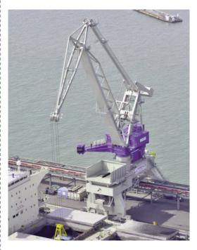
Minimized energy consumption is based on a purely electric operation with the associated high energy-efficiency advantages. The jib system geometry provides a balanced system with anti-friction bearings fitted to the pivot points. Energy losses from the movement of dead loads, which occur in the jib system of single jib cranes and the trolley of ship unloaders, are avoided. Energy recovery units are installed on all Ardelt cranes as standard.
