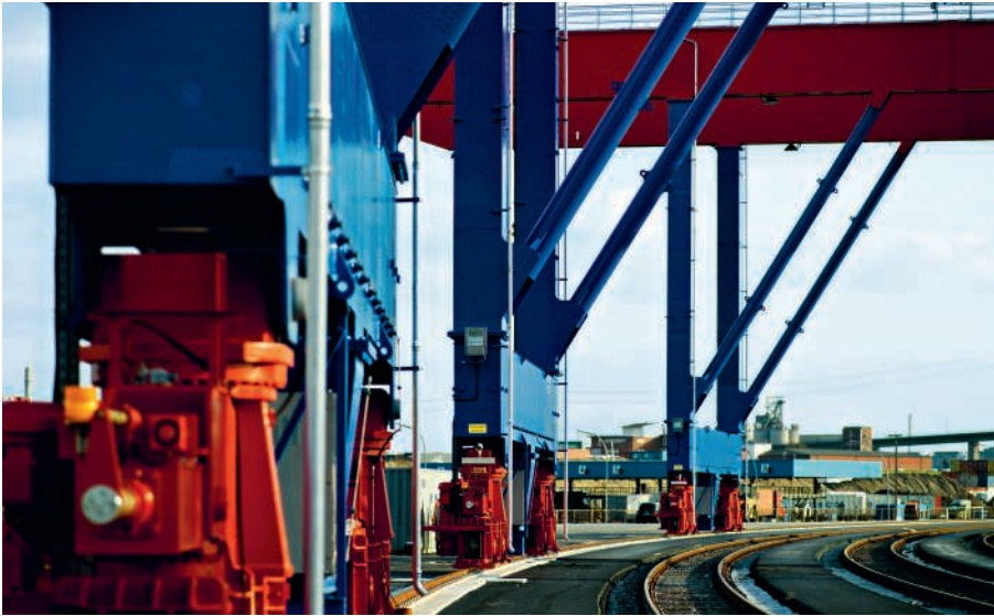
↑ Option: slewing gantry travelling mechanism
